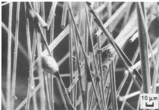
Figure 13 Micrograph showing the widespread nature of the formation of the "spheres".
